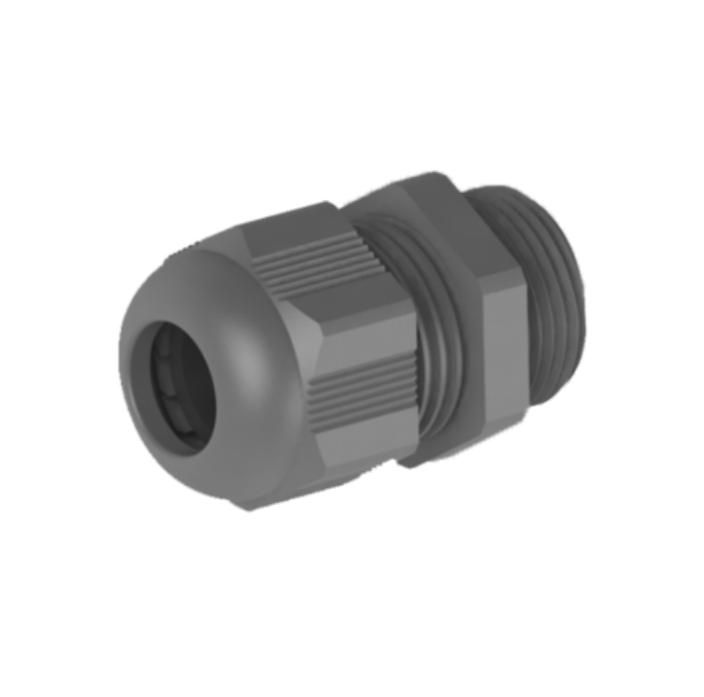
**MOREK PRESETUPA, M32, 18-25MM, PA6, GREY RAL7001, IP68 (W LOCKNUT AND O-RING)**
