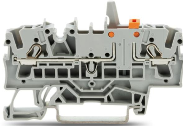
**WAGO 2-CONDUCTOR DISCONNECT/TEST TERMINAL BLOCK; WITH MECHANICAL INTERLOCK; WITH TEST OPTION; ORANGE DISCONNECT LINK; FOR DIN-RAIL 35 X 15 AND 35 X 7.5; 2.5 MM<sup>2</sup>; PUSH-IN CAGE CLAMP®; 2,50 MM<sup>2</sup>; GRAY**
