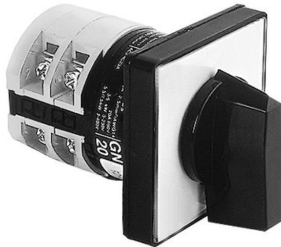
**LOVATO INTRERUPATOR ROTATIV CU CAME, GN SERIES, U VERSION, FRONT MOUNT. VOLTMETER SWITCH, FOR 3 PHASE TO PHASE TENSIUNE AND 3 PHASE TENSIUNE READINGS - 3 WAFERS – SCHEME 66, 16A**
