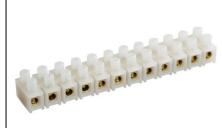
Applied for screw connection of conductors, protecting wires from damage and excluding possibility of short circuit to the frame of electric unit. Insulation frame is made of white non-flammable polystyrene or transparent polyethylene. Terminal block and screws - latten alloy. Protection of the wire from damage and exclusion of the possibility of a short circuit to the housing of the electrical installation.
