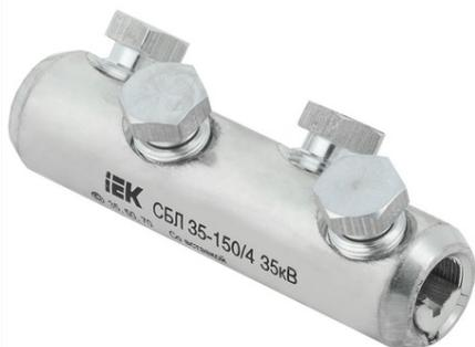
Universal galvanized cable end sleeves with shear heads. Designed to connect any type of cable cores up to 35 kV: aluminum and copper, round and sector, solid and stranded. For any type of cable cores: aluminum and copper, round and sector, solid and stranded.
