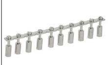
Jumpers (combs) are used for the electrical connection of rows of screw-type terminal assemblies (KWI terminals) in distribution systems. They are installed in the center of the terminal in the corresponding grooves of the current-carrying plates by screwing the connecting screw into the busbar. Made as steel plates with 2, 3 or 10 leads.Rated operating current and voltage: 24 to 85A / up to 800V.
